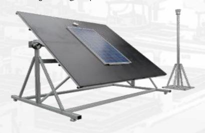
Temperature test for IEC 61730 & UL 1703 also in here carry out. We provide 19mm thick wood (current standard) or a thermal insulation with a k factor ≤0.24W/m2K (IEC 61730 Ed.2) black painted wooden platform, the platform is to extend at least 0.6m beyond the module on all sides, can fast loading.
