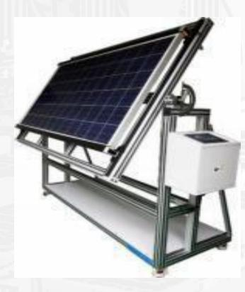
Incidence angle automatic positioning device (IEC 61853-2) For IEC 61853-2:2016 energy rating – Incidence angle and module operating temperature measurements
